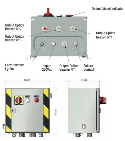
\* The visual elements are for guidance only. The size of the power supply control panel can change depending on the options needed.
